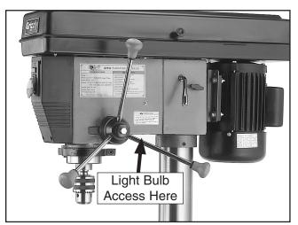
Figure 21. Light bulb access location.
